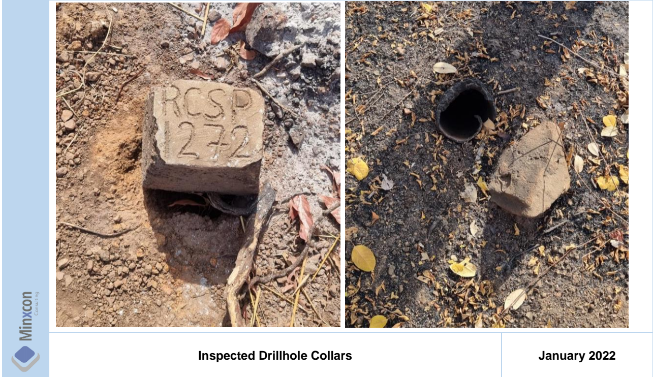
Figure 1: Inspected Drillhole Collars
