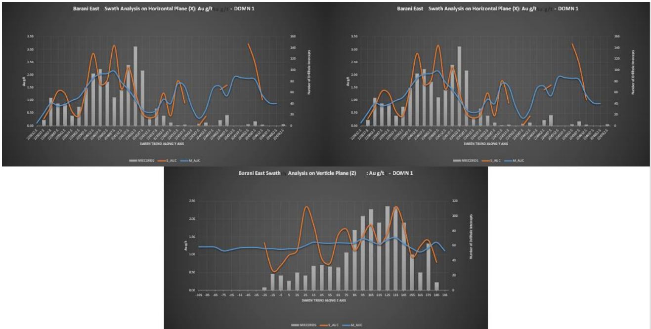
Figure 140: An Example of a Swath Analysis Comparing the Ordinary Kriged Estimate (Au g/t) with the Average Value (Au g/t) of Composites in Various Orientations through the Estimated Block Model for Barani East
