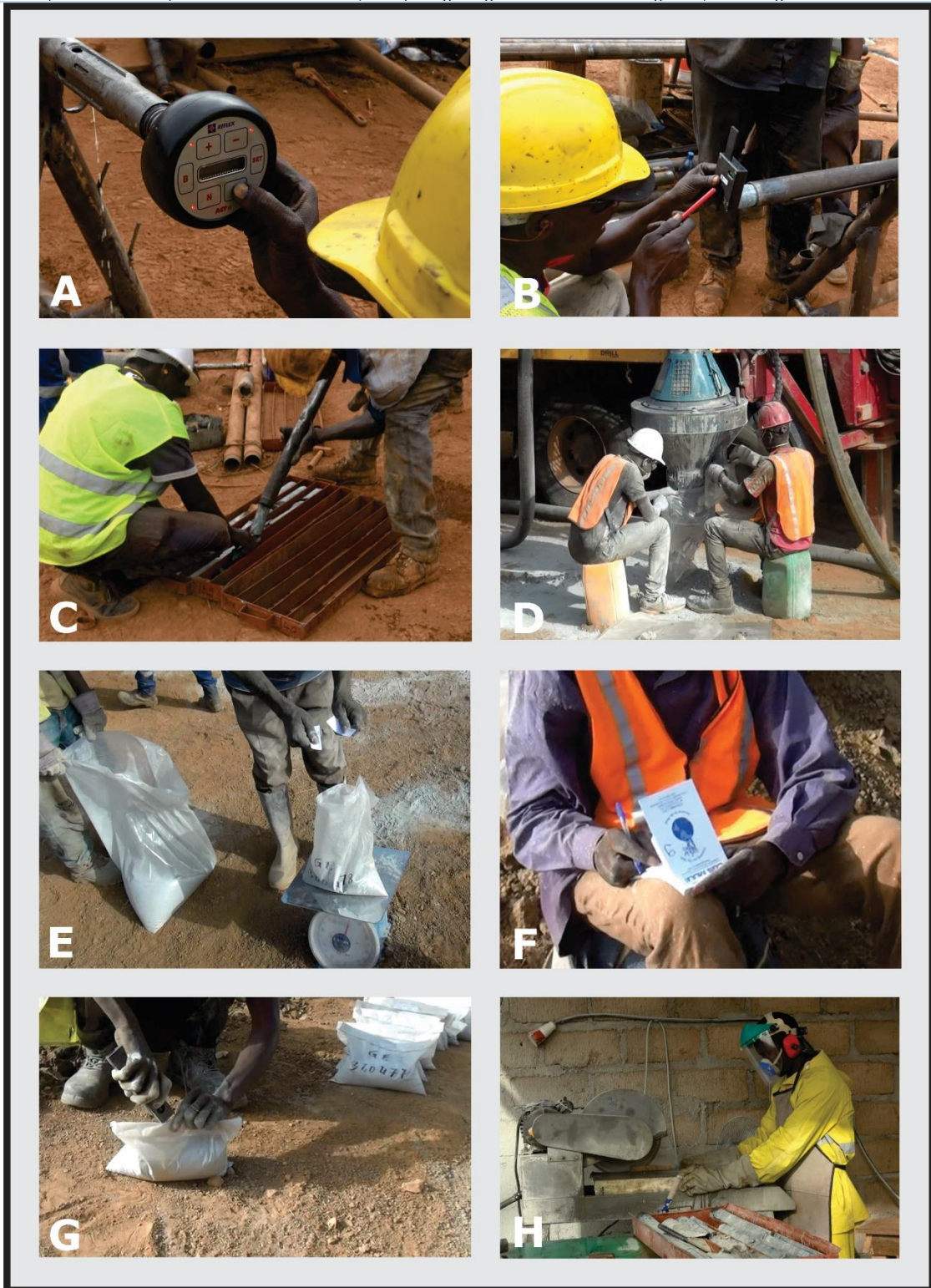
Figure 77: Photos of Drilling and Sampling Procedures. A) Collecting Reflex Act II oriented core readings and resetting the instrument; B) marking the core for orientation C) removing core from the core barrel into core trays; D) collecting samples at the RC cyclone; E) weighing samples; F) recording sample information in printed sample ticket books; G) stapling bags closed with tags; H) sawing core.
